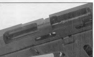
Glock Model 30 .45 ACP (top) and Model 29 10mm Auto (bottom), right-side view. (inset) Unique factory cutaway shows the Glock's spring-loaded firingpin safety blocking the striker's forward movement. made from .401 Winchester Self-Loading Rifle semi-rimmed cartridge cases cut back to a length of 1.25 inches. It remained a wildcat, and interest quickly waned.
